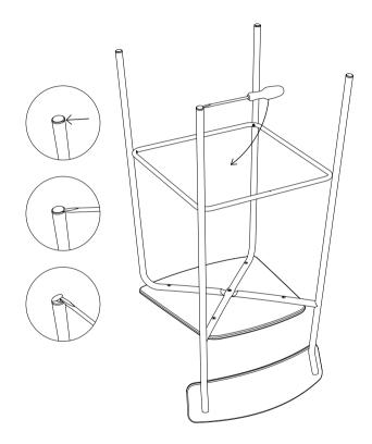
You can later exchange the glider by placing screwdriver in groove and push down
