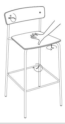
Push down on seat and tighten all screws
