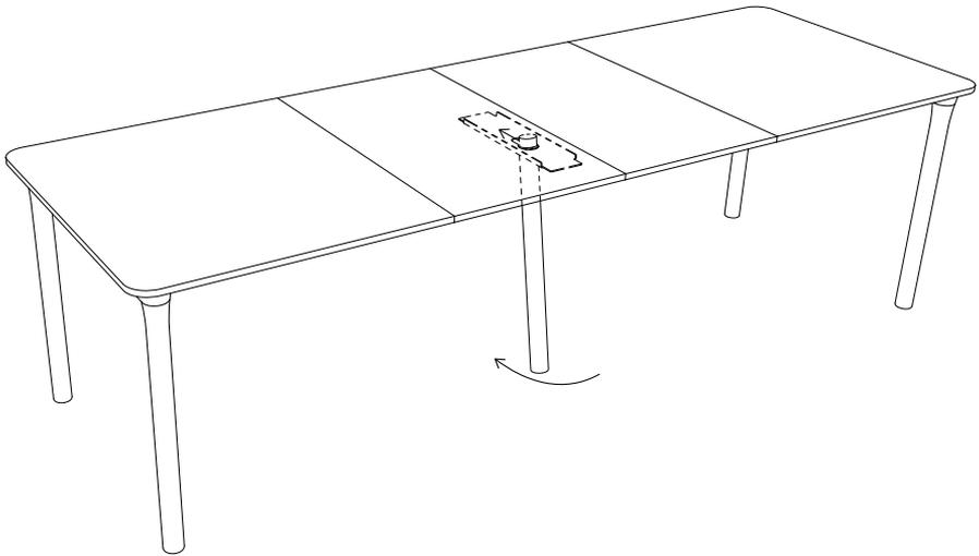
Fit the support leg in the metal bracket. Slide the leg along the keyhole in the bracket by the groove in the leg.
